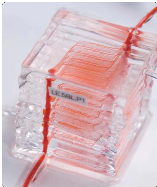
FIGURE 2 A multilayer PDMS microfluidic oxygenator for artificial lung applications. Each of the ten layers of the device comprises a microvascular network and an oxygen delivery compartment separated by a thin (11 \mu\text{m} ) membrane.
