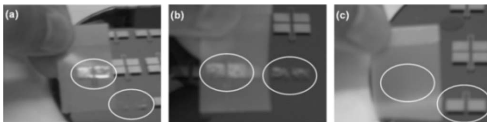
Fig. 3 Results of the Scotch tape test of gold patterns embedded in PDMS: (a) no treatment, (b) treatment with 3-mercaptopropyltrimethoxysilane vapor, and (c) treatment with 20 mM 3-mercaptopropyltriethoxysilane in isopropyl alcohol.
