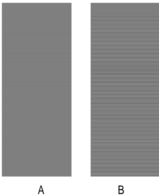
Figure 2. Comparison between a A normal printout and B a printout with banding. Both printouts are printed with 25% fill.
