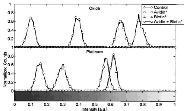
**Figure 4.** Histograms of fluorescence emission from the chip surfaces of a reference unprocessed chip, avidin adsorption, biotin adsorption, and avidin biotin reaction. Histograms labeled “control” correspond to untreated surfaces. An asterisk next to a particular species indicates that there is a fluorescent label attached to it.
