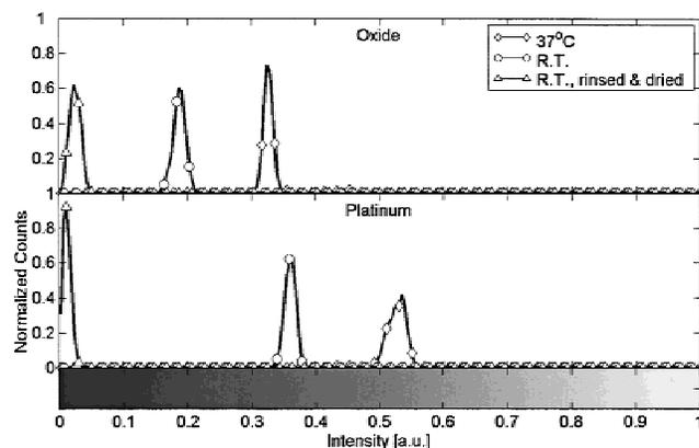
**Figure 2.** Histograms of fluorescence emission of fluorescein-labeled avidin from the chip surfaces under incubation at room temperature (RT) for 15 h, incubated at 37°C for 15 h, and when the chips were rinsed in DI and dried. Highest emission coincides with peaks on the right of the intensity scale.
