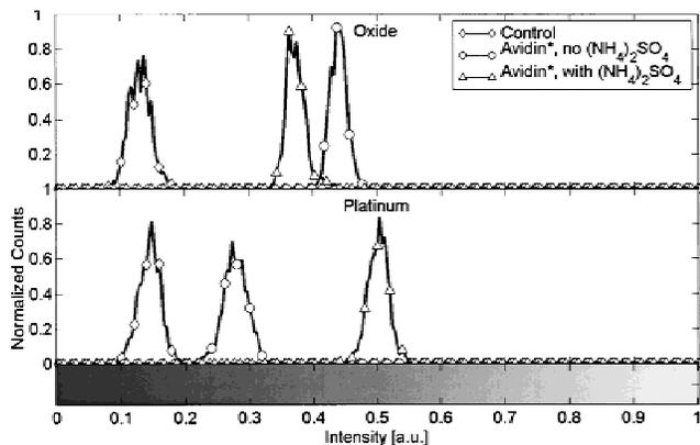
**Figure 3.** Histograms of fluorescence emission from the chip surfaces of a reference unprocessed chip, avidin adsorption at 37°C for 15 h, and avidin adsorption using ammonium sulfate precipitation. The histograms labeled “control” correspond to untreated surfaces. An asterisk next to a particular species indicates that there is a fluorescent label attached to it.
