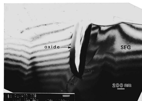
FIG. 10. TEM micrograph of the reoxidized diode showing the dramatic reduction of defects in the SEG.
