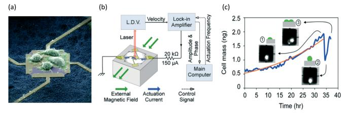
Fig. 3 Pedestal Resonant Sensor. (a) Cells are cultured on a platform for the mass measurements. (b) The phase of the velocity was measured with a laser Doppler vibrometer to extract the changes of resonant frequency and thus cell growth. (c) The change of the single cell mass was obtained with cell imaging. The cell mitosis event was reflected as a sharp decrease on the cell growth profile (adapted and reproduced with permission from ref. 26).
