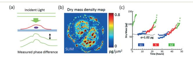
**Fig. 1** Optical measurements of cell mass and growth. (a) In quantitative phase imaging the path length delay of light travelling through a cell is measured as a phase difference which is directly proportional to the dry mass density of the cell at each point in the image. (b) Dry mass density map. (c) The growth characteristics measured with PCNA cell cycle reporter (adapted and reproduced with permission from ref. 19).
