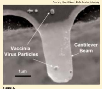
Electron micrograph of individual virus particles on a cantilever
